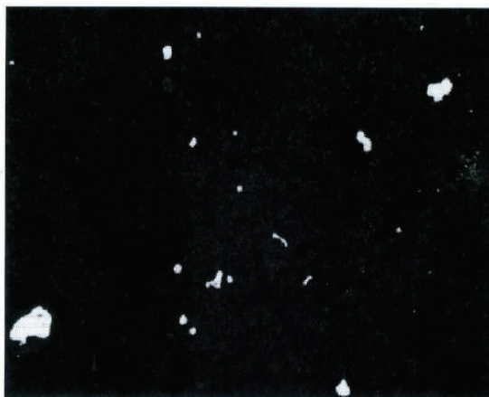
Fig. 3.1 Microstructure of aluminium-aluminium oxide composition at 0.05 % of aluminium (The photograph was made in polarized light)
